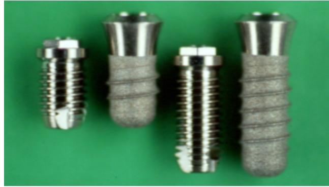
Figure 1. Commercially available Brånemark and Straumann implants used in this study. From left to right, 7 mm Brånemark, 6 mm ITI, 10 mm Brånemark and 10 mm Straumann implants.
