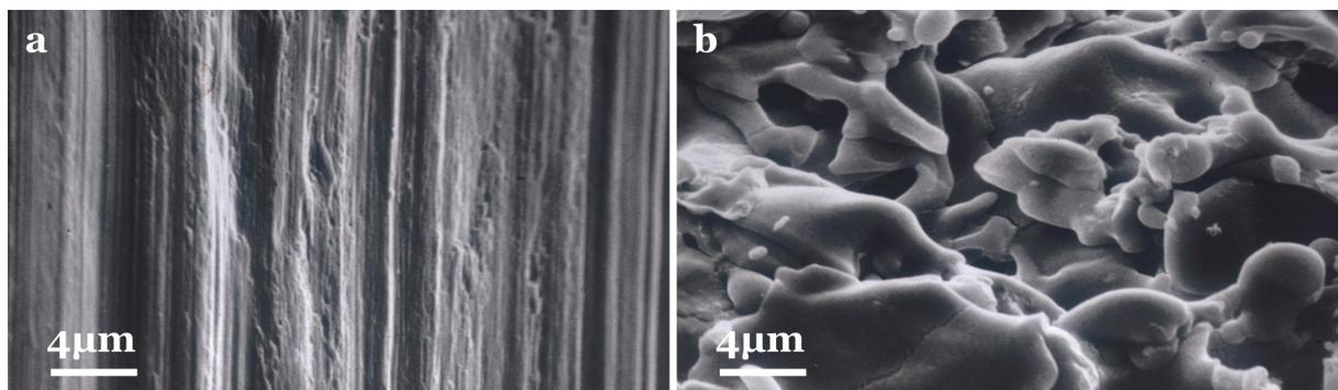
**Figure 2. Scanning electron microscopy micrographs of the implants surfaces.** (a) Brånemark fixture, the surface feature corresponds to the machining grooves (x 3000). (b) Straumann implant, the surface is roughened by titanium plasma-spraying (x 3000).
