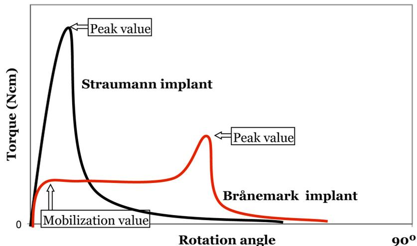
**Figure 3. Schematic representation of the loosening modes of the 10 mm long Straumann and Brånemark implants.** Note the mobilization torque level for the Brånemark implants, the plateau attained during the rotation phase, the peak-value and the steep decrease of the reverse-torque value.
